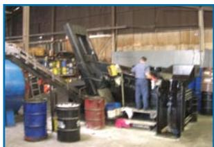
Squeeze about 100,000 gallons of oil from nearly 10,000 drums of filters annually.
