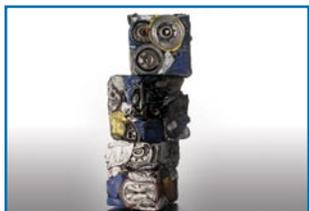
Filters after cubing and oil extraction.
